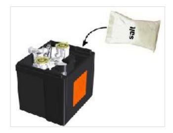
3. Add water in the salt container until the water level is approx. 4" high. (the float on the brine valve must be afloat)
