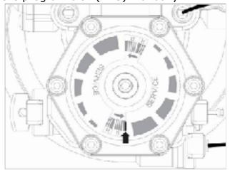
Turn Regeneration Disk counter clockwise until it is in above position. When the arrow and the small line on the transparent cover reach the area marked by "B" (brining), a regeneration will start. Immediately, the Regeneration Disk will drop down a little (you will be able to see and hear this).
