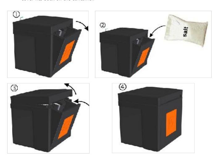
Note: Watch carefully that you don't squeeze the tube when opening or closing the tilt drawer for the salt.
