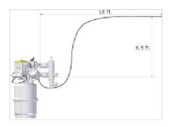
Note: Maximum height and distance of flexible drain hose
